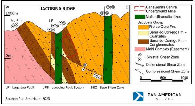
Figure 7-6: Generalized cross-section through the Canavieiras Central Mine
