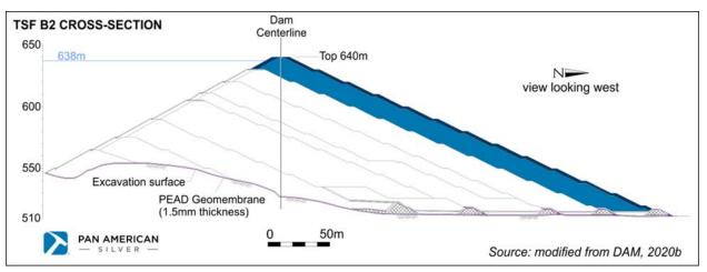
Figure 18-2: Cross-section of TSF B2 dam at final elevation
